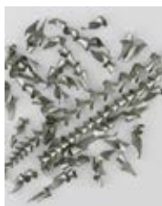
Material: SS304 Ø8mm / depth 16mm Vc = 20m/min f = 0.15mm/rev
