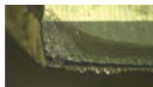
Competitor A Hole 600 Wear = 0.03mm
