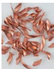
Material: Cu Ø8mm / depth 5mm Vc = 40m/min f = 0.15mm/rev
